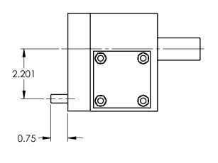
PAWL SHAFT MOVES 7° BETWEEN INDEX AND RESET (CAM DRIVEN AT RESET AND SPRING DRIVEN AT INDEX. USE NON-CONTACT SENSOR ONLY).
